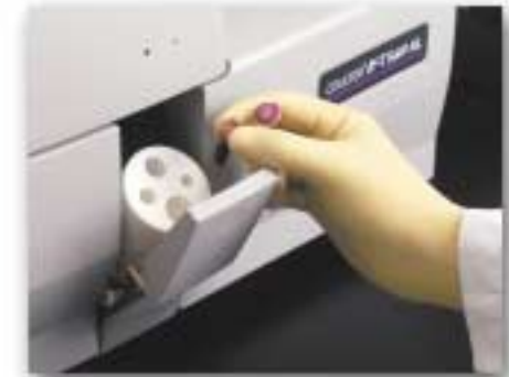
Two additional tube holders accommodate tubes of varying sizes.
