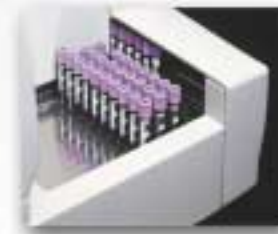
The AC•T 5diff AL has 100 sample loading capacity.
